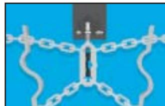
Hook in the connecting hook into the synthetic bow, fasten it with the screw and the nut and insert the safety clip.
