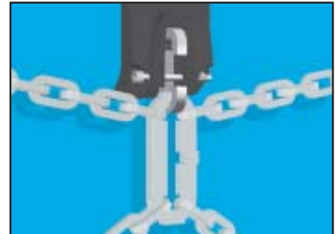
Adjustment joint in position "short" (across to direction of driving)
