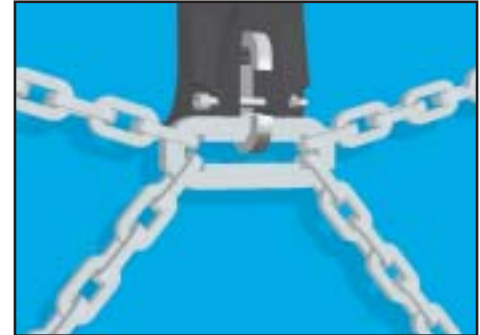
Adjustment joint in position "long" (in direction of driving)
