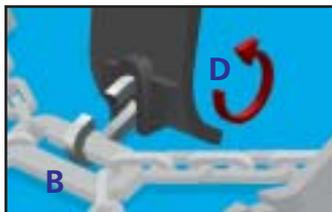
Tilt the synthetic bow (D) towards the adjustment joint (B) and remove the synthetic bow.
